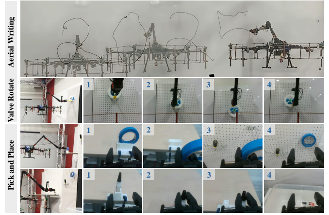
Fig. 8. Aerial Teleoperation Manipulation Tasks. We target 1) Aerial Writing: UAM with a marker pen writes ‘2025’ on a whiteboard. 2) Rotate Valve: UAM grasps the handle and rotates the valve with one loop. 3) Pick-and-Place: UAM grasps an object and relocates it to a designated area.
